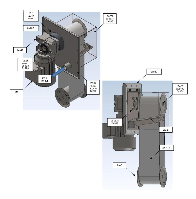
Fig. 2a view of oil skimmer components (pos. 2a-1)
