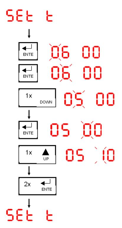
Figure 6.3.2-9 Illustration of the procedure for entering the date and time
