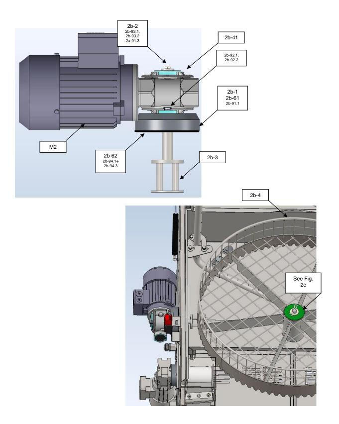
Fig. 2b view of basket drive components
