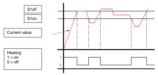
Figure 6.3.2-4 Illustration of heating element switching
