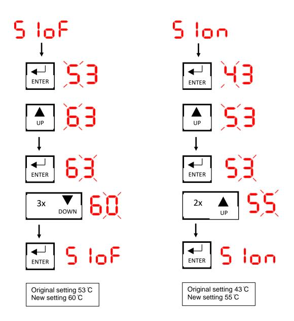
Figure 6.3.2-3 Illustration of the procedure for setting of parameters (temperature)
